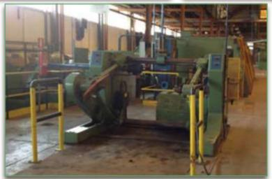
Detorsion Conic Laying Up DE ANGELI 3+1 Ø1200, Capstan Ø2000, Taping head diam. 500mm for paper and PVC. Take Up DE ANGELI Ø2000
