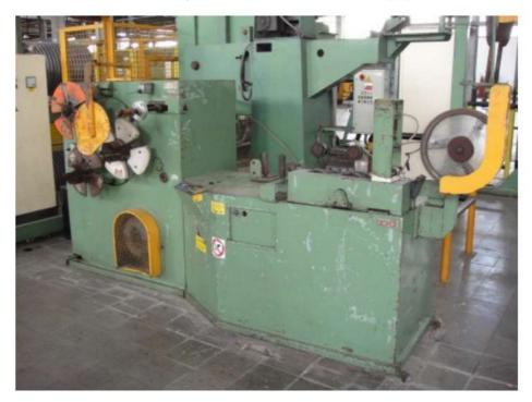
• Coiling machine DE ANGELI MD2, 2 head Ø560x180
