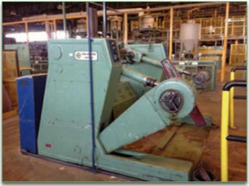
Armouring line 120 wires DE ANGELI, suitable for bobbins diam. 200mm, PayOff 2200, armouring head with 2 pads Ø500, taping head with 3 pads Ø500, Caterpillar 1200mm and Take Up.
