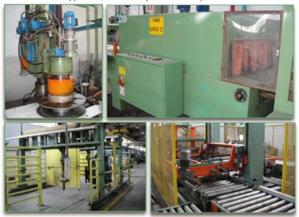
Paper box down coiler machine BRIANTECH F500 for carton box from 320 to 520mm of diameter and with height from 400 to 800mm. Range of cable diameter: from 1.2 to 6 mm
