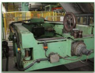
Drum Twister 2200 with 3 rotating PayOff Ø1600, rotating PayOff 2200, rotating TakeUp 2200, Caterpillar complete of all loading platforms, taping and armouring heads.
