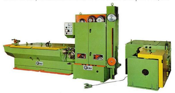
Intermediate drawing machine ROBERTSON 13P, 13 dies, 300 mm diameter capstan, AC or DC motors. Annealer. Available with Spooler 630 DIN. Outlet diameters up to 2.50 mm. Max speed 20 m/sec.
