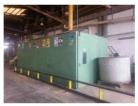
Electrolytic tinning line suitable to tin copper wires with diameter from 1,00 to 3,00 mm, raw and baked copper wire. It is also possible to obtain tinned wires with diameter of 0.80 mm because tinned wires can be redrawed.
