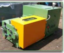
Prawing machine SAMP TRB 4, 21 dies, tungsten carbide capstan, AC or DC motors. Annealer. Available with Spooler 400 DIN. Inlet diameter: 1.6 mm, Outlet diameters from 0.10 to 0.3 mm. Max speed 35 m/sec.
