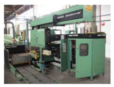
Coiling machine TECNOMATIC, n.°2 portal Pay Off Ø1600, Vertical accumulator Ø500, Coiling head Ø600x220mm, coil height 250mm, with strapping machine, heat shrink film applicator, automatic palletizer and packer.
