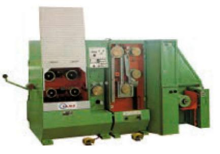
Drawing machine SAMP TRB 5, 21 dies, tungsten carbide capstan, AC or DC motors.
