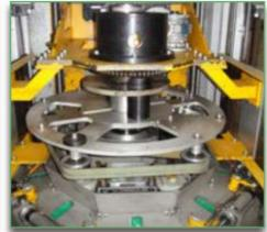
Coiling machine DE ANGELI MD, 3 head Ø400x160x130(h)
